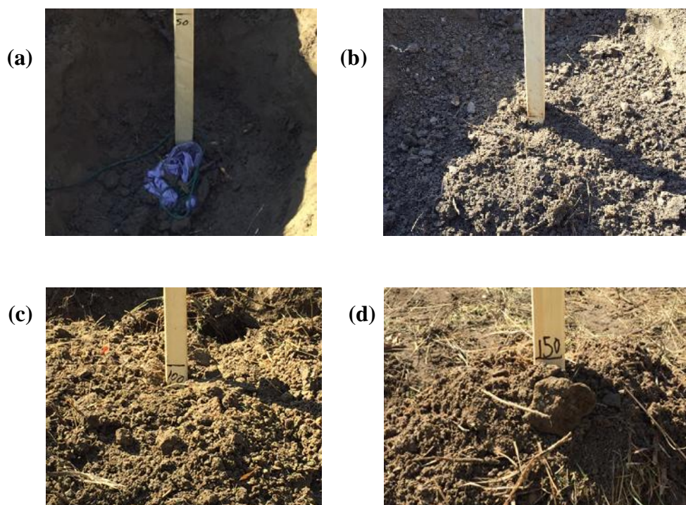
Figure 2.11. Deposits refilled to various heights: (a) 0.0 m, (b) 0.5 m, (c) 1.0 m, and (d) 1.5 m.
