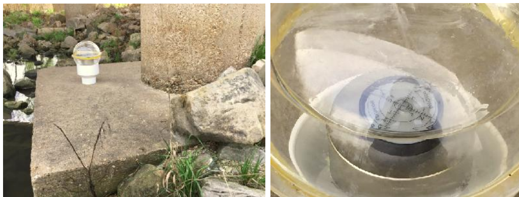
Figure 2.13. The APUS prototype placed on a bridge footing.
